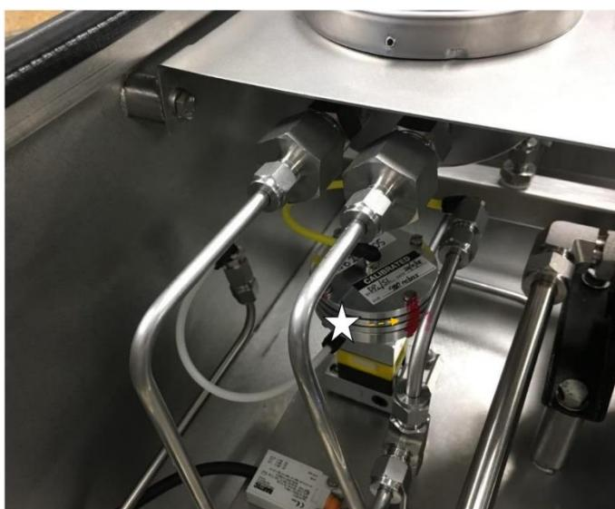
2. Firmly grip the sensor alloy housing with your hand and rotate anticlockwise to unscrew the sensor from the base (yellow block).
