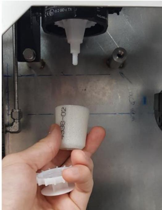
3. Replace with the new element and push the bowl back up and twist until it is set back in place.
