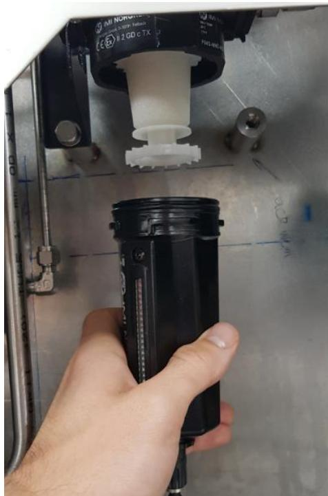
2. Remove the filter element by unscrewing it.
