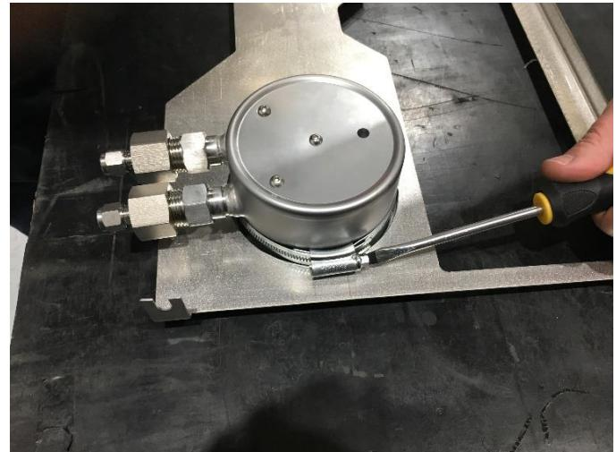
7. Tighten the 4 hex screws and the nuts on the gauges.
