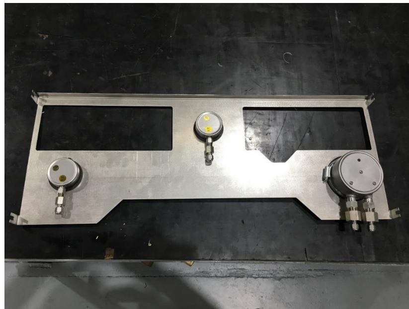
4. Use circlip pliers and remove the circlip holding the gauge onto the chassis plate. If it is the larger DP gauge, there will be a hose clip holding it on. Unscrew the hose clip and remove the gauge.
