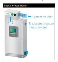
After the purge step is completed, the pressurization control system supplies sufficient air to maintain a constant overpressure inside the pressurized enclosure, compensating for any small leaks, and preventing the ingress of the outside atmosphere. The enclosure pressure is monitored. The enclosure contents can be energised.
