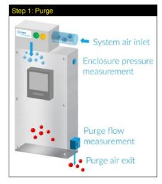
The pressurization control system supplies clean, dry instrument air to the pressurized enclosure at a high flow rate for a pre-set time, expelling any potentially flammable atmosphere remaining inside through an outlet valve. Enclosure pressure and purge air flow are monitored. The enclosure contents are not energised.
