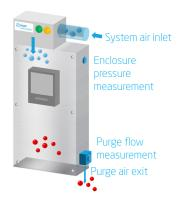
**Purge:** The purge system supplies clean, dry instrument air to the enclosure at a high flow rate for a pre-set time, expelling any potentially flammable atmosphere remaining inside. Enclosure pressure and purge flow are monitored. The electrical equipment inside the enclosure is not energised.
