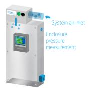
**Pressurization:** After purge is complete, the system supplies sufficient air to maintain a constant pressure inside the enclosure, compensating for any small leaks, preventing ingress of the outside atmosphere. Enclosure pressure is monitored. The electrical equipment inside the enclosure can be energised.
