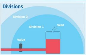
The classification of Zones and Divisions is related to the frequency and duration that ignitable gases or dusts may be present in the atmosphere.
