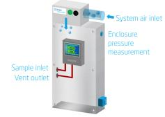
Analyser installation: Introducing a sample gas or liquid into the enclosure becomes an important consideration. For non-flammable samples, there is generally no issue. For flammable samples, a leak may cause a dangerous situation if it comes into contact with live electrical equipment.
