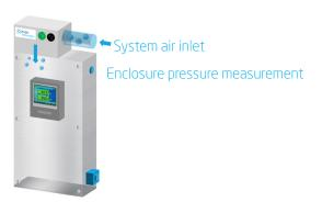
**Pressurization:** After purge is complete, the system supplies sufficient air to maintain a constant pressure inside the enclosure, compensating for any small leaks, preventing ingress of the outside atmosphere. Enclosure pressure is monitored. The electrical equipment inside the enclosure can be energized.
