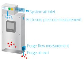
**Purge:** The purge system supplies clean, dry instrument air to the enclosure at a high flow rate for a pre-set time, expelling any potentially flammable atmosphere remaining inside. Enclosure pressure and purge flow are monitored. The electrical equipment inside the enclosure is not energized.
