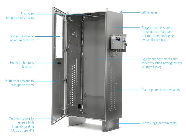
The system shown here, prior to customer fit-out, is equipped with an Expo MiniPurge and interface unit to provide Class I Div.1 protection, with power & signal control.
