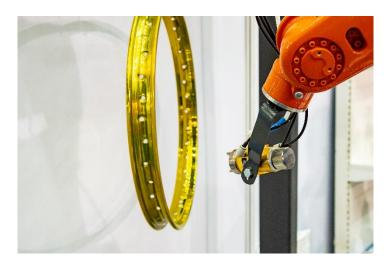
Painting robots apply coatings with great precision and evenness and are increasingly a feature in many manufacturing environments. In particular, the automobile industry has used painting robots for many years.
